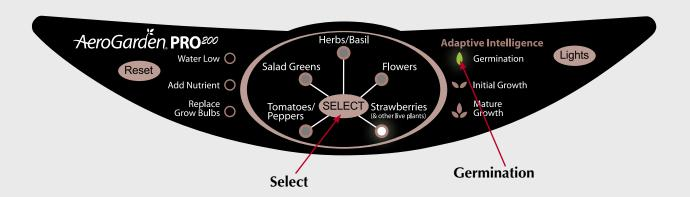
Once your AeroGarden PRO<sup>200</sup> is set on the "24-Hour Light" setting, the lights and pump will remain on 24 hours a day. To shorten the amount of time lights are on, quickly press and release "Lights" button, and lights will turn off. Lights will automatically come back on within 12 hours – or, you can press and release "Lights" button again, to turn lights back on.
